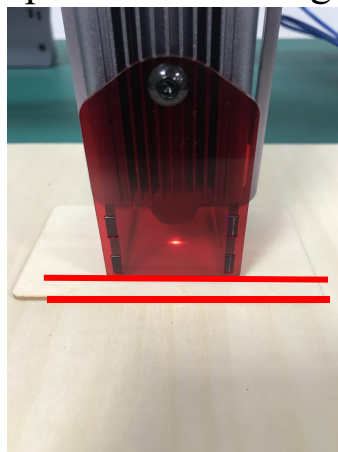
Picture 4.2 The shield is parallel to the edge of the engraved object
